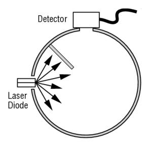
*Figure 2* 819D integrating sphere configuration.
