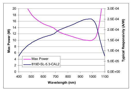
Figure 5 Typical responsivity curve of 819D-SL-5.3-CAL2
